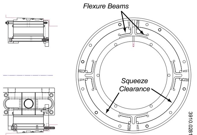
Fig. 3. Squeeze film damper used for bearing support
