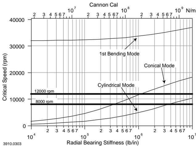
Fig. 2. Undamped synchronous critical speeds as a function of support stiffness, for the CCEML compulsator rotor
