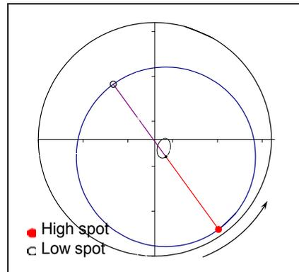
Figure 2. Journal and bearing with exaggerated clearance. Journal center and orbit calculated at 3975 rpm with 25.2 kg-mm imbalance. Journal instantaneous position is at moment of minimum film thickness.
