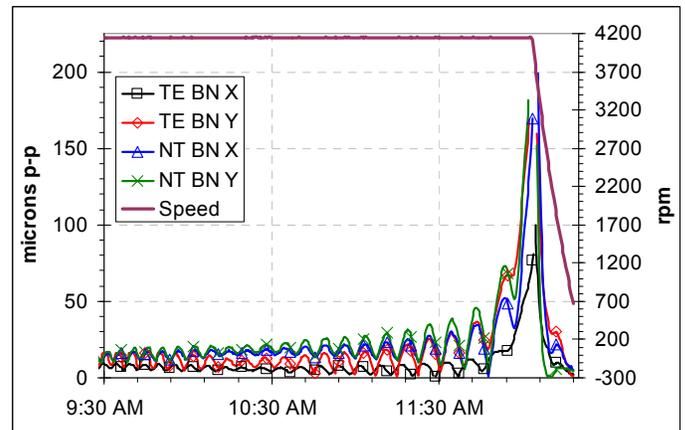
Figure 8. 4150 RPM Constant Speed Factory Test of Unit 2 – Prox Probes 1x Vibration Amplitude vs. Time.
