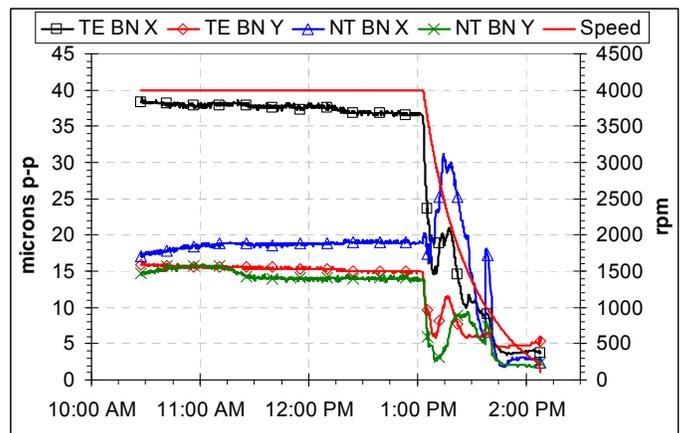
Figure 24. 4000 rpm Factory test of Unit 5, new 4 lobe bearing – prox probes 1x vibration amplitude vs. time.
