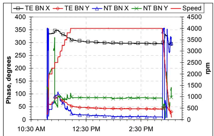
Figure 22. 4000 RPM Constant Speed Factory Test of Unit 4 with New 4 Lobe Bearing – Prox Probes 1x Phase
