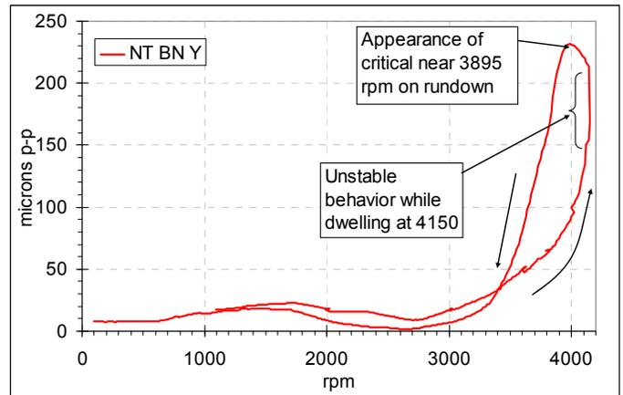
Figure 10. Unit 1 – Appearance of Critical Speed at 3985 RPM at Run-down from 4200 RPM.
