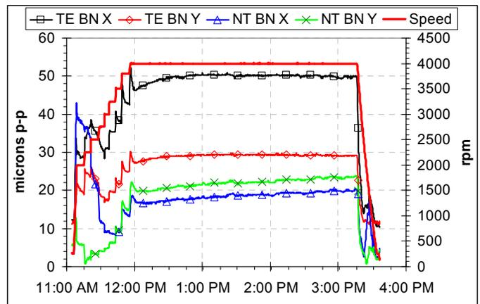
Figure 21. 4000 RPM Factory test of Unit 4, new 4 lobe bearing – prox probes 1x vibration amplitude vs. time.
