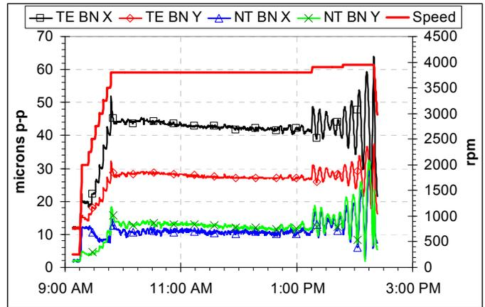
Figure 23. Factory test of Unit 4, original partial arc bearing (3800→3900→3950 rpm) – prox probes 1x vibration amplitude vs. time.
