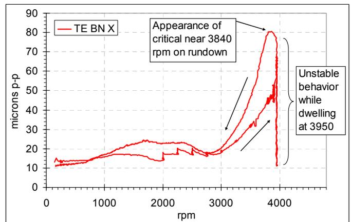
Figure 12. Unit 4 – Appearance of Critical Speed at 3840 RPM at Run-down from 3950 RPM.
