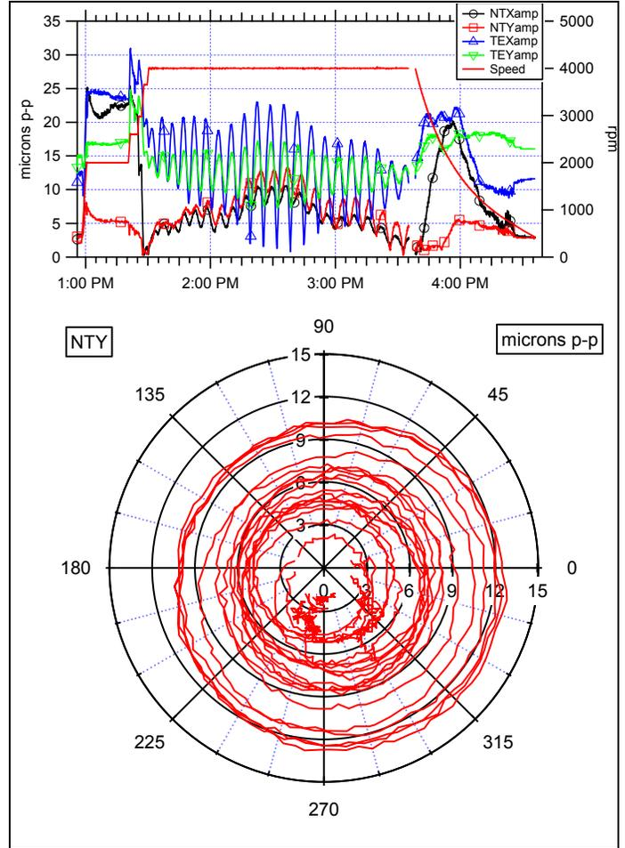
Figure 14. Unit 3 – Oscillatory Behavior at 4000 rpm.
