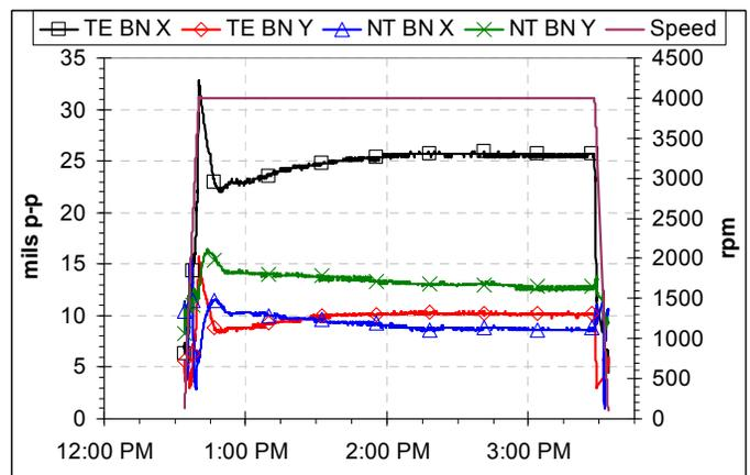
Figure 25. 4000 RPM Factory test of phase 2 Unit 2 with modified 4 lobe bearing – prox probes 1x vibration amplitude vs. time.
