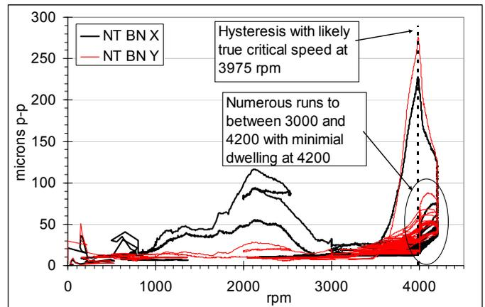
Figure 11. Unit 1 – Appearance of Critical Speed at 3975 RPM at Run-down from 4200 RPM – Off-Site Testing.
