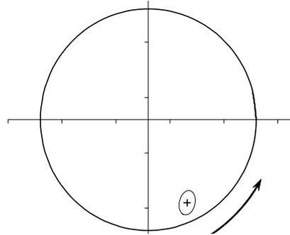
Figure 1. Bearing clearance circle and 1X orbit calculated at 3975 rpm with 25.2 kg-mm imbalance. Orbit is centered at static eccentricity position calculated with bearing code.
