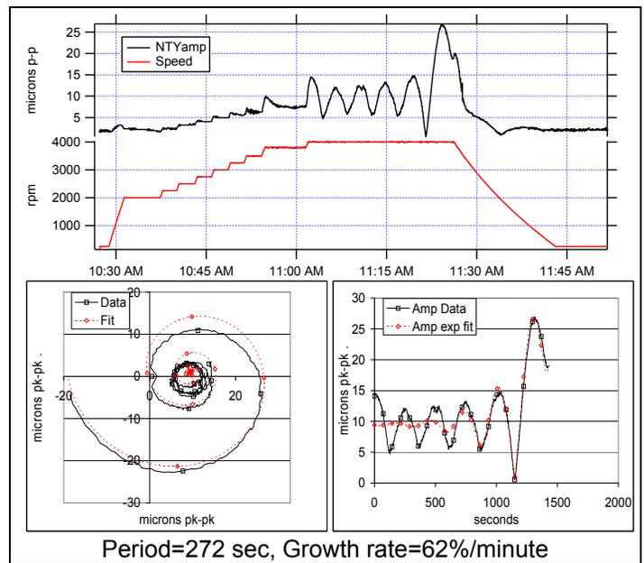
Figure 17. Unit 4 – Event 10 – More Rapidly Diverging Spiral Vibration Behavior at 4000 rpm.
