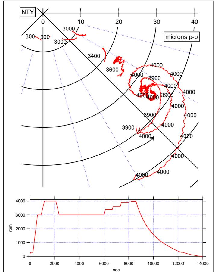
Figure 16. Unit 1 – Converging Spiral Vibration Behavior at speeds from 3000 to 4000 rpm. Labels on curves are rpm.
