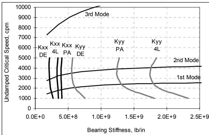
Figure 20. Synchronous undamped critical speed map as a function of bearing stiffness, with bearing stiffness data. DE=drive end PA bearing. PA & 4L are for NTE bearing.
