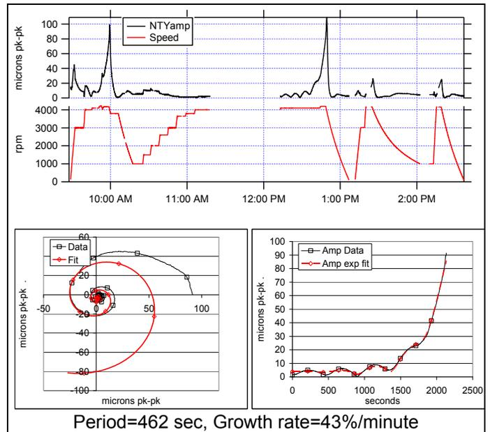
Figure 15. Unit 3 – Divergent Spiral at 4100 rpm.
