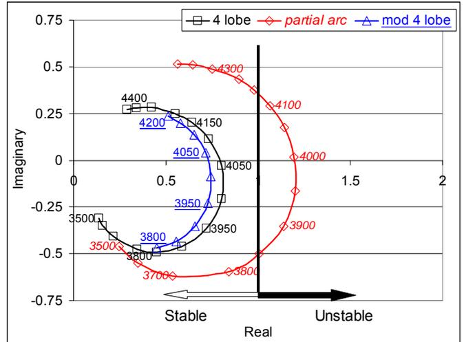
Figure 18. Morton Effect stability plotted in the complex plane – original partial arc bearing, 4 lobe bearing, and modified 4 lobe bearing. Labels on curves are rpm.
