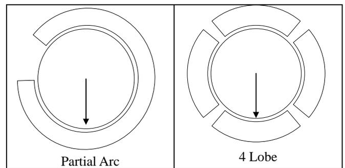
Figure 3. Schematics of tested bearing configurations.
