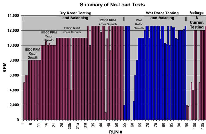
**Figure 4. Summary view of No-Load testing phases**
