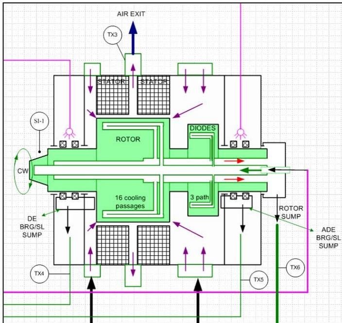
**Figure 1. ALPS HS-Generator lubrication and cooling schematic**
