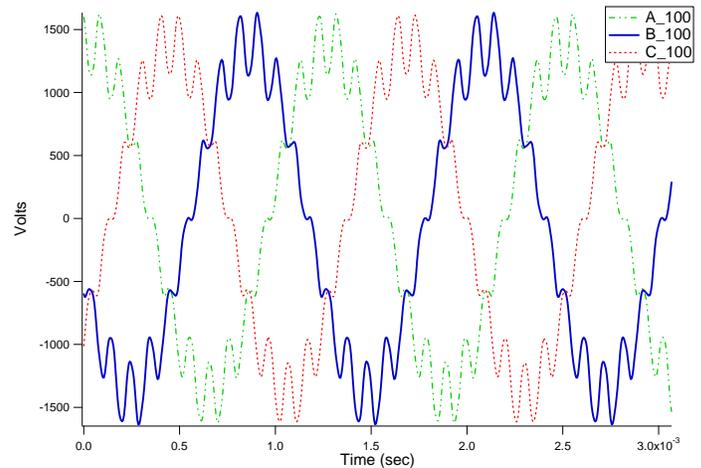
**Figure 5. Three phase open circuit voltage waveform**
