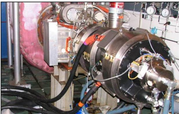
**Figure 7. View of high-speed generator installed in turbine test cell with ETF40B engine**
